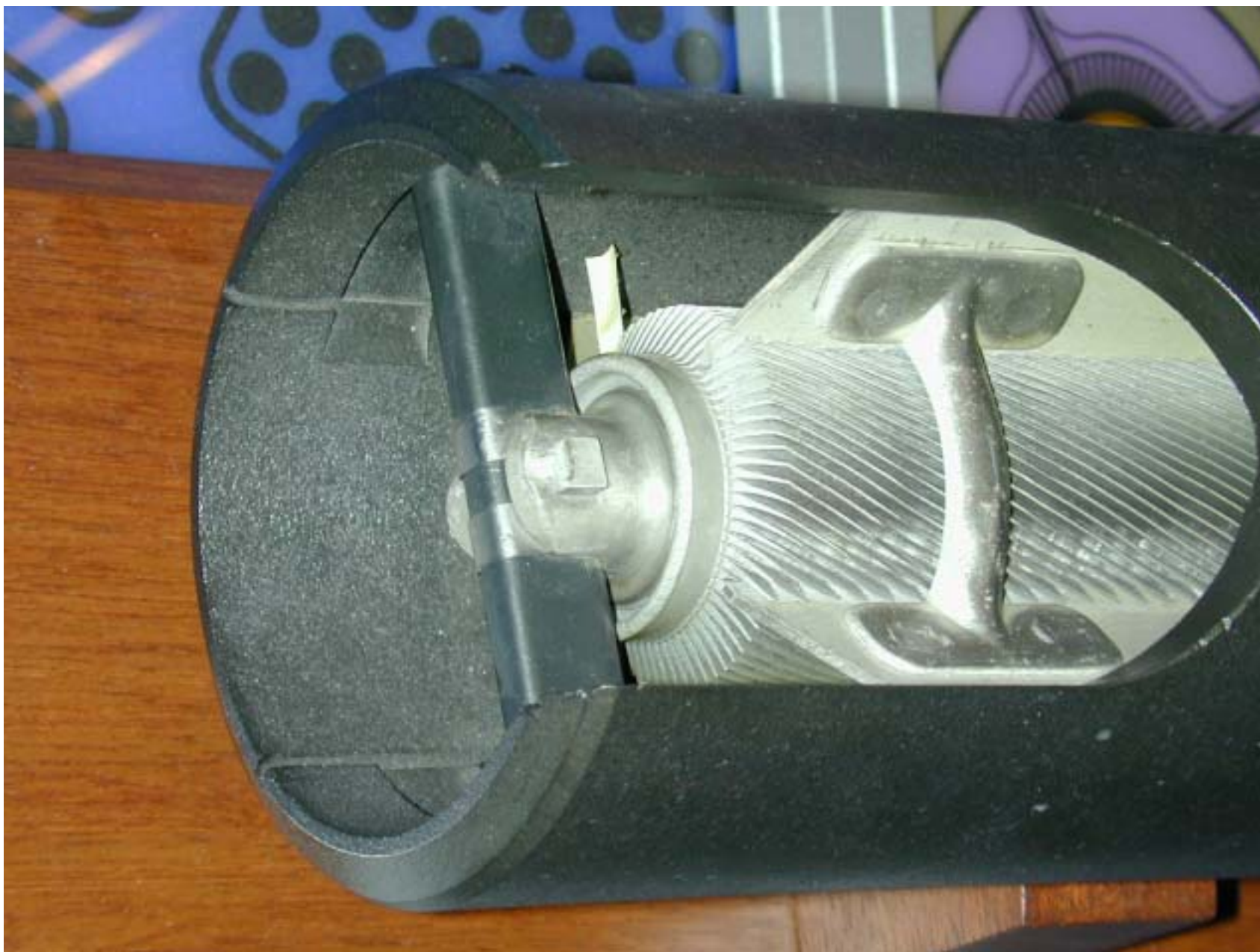
Fuel element of graphite-moderated gas-cooled reactor (from the bottom)
